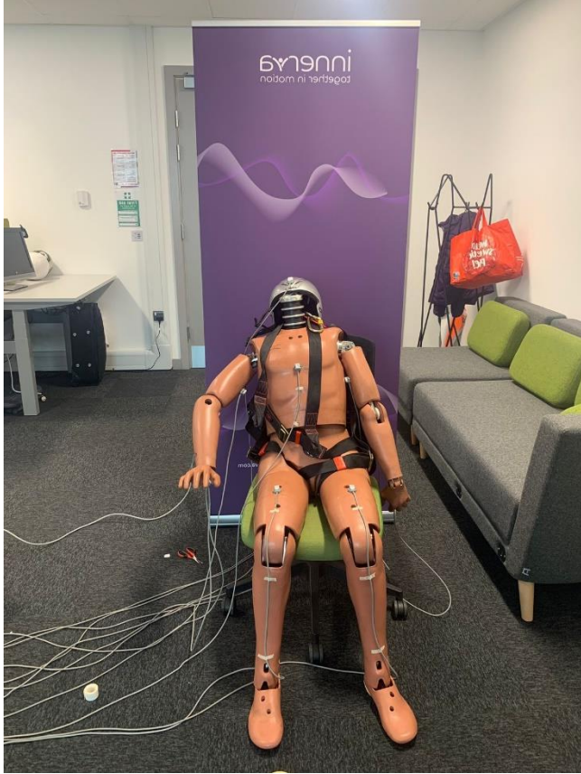
Figure 9: i) Crash test dummy instrumented with motion capture sensors ii) Areli instrumented during an experiment iii) Areli outside the AWRC
